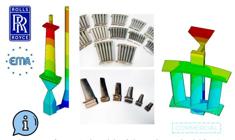
Development of numerical models of the cooling and solidification steps in Directional Solidified ("DS") and Equiax ("EXQ") investment casting processes
